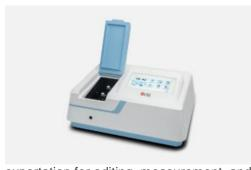
The instrument is equipped with a 10.1-inch large color touch screen (1024\*600), designed with an easy-to-use graphical user interface.
